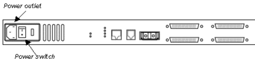
Figure 11. PowerVault 35F power switch and outlet
